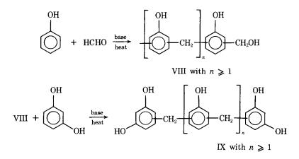
Compound IX is then mixed with untreated flavonoid polymers to form an adhesive that can be set at ambient temperature by addition of paraformaldehyde.
