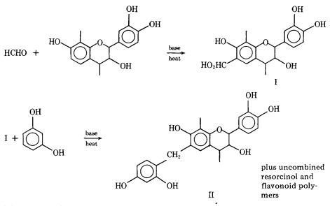
Mix II is an adhesive that can be set at ambient temperature by addition of paraformaldehyde.
